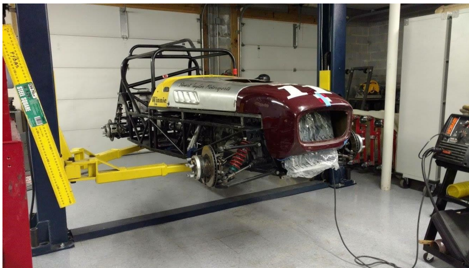
Fitting old body panels to the new higher upper subframe for clearance of the new F20c
